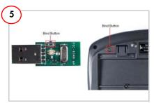
Press the bind button on the bridge; the red LED blinks. Press the bind button on the keyboard to bind it with the bridge. The mouse and keyboard work smoothly with the PC.
