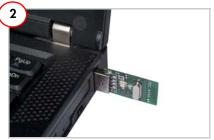
Connect the bridge dongle to the PC. The bridge enumerates as a human interface device (HID).
