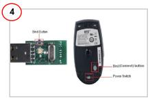
Turn on the mouse. Press the bind button on the bridge; the red LED blinks. Press the bind button on the mouse to bind it with the bridge.
