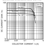
Fig.1 DC current gain vs. collector current
