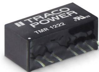
The TMR-2WI series is a new family of isolated 2W dc-dc converter modules with regulated output, featuring ultra-wide 4:1 input voltage ranges of 9-36 VDC or 18-75 VDC. The product comes in a ultra-compact SIP-9 plastic package.
