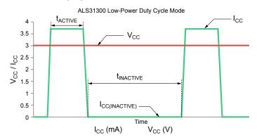
Figure 4: I<sub>CC</sub> in Low-Power Duty Cycle Mode
