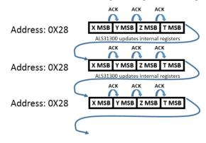
Figure 7: Fast Loop Mode
