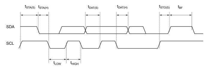
Figure 3: I<sup>2</sup>C Interface Timing Diagram
