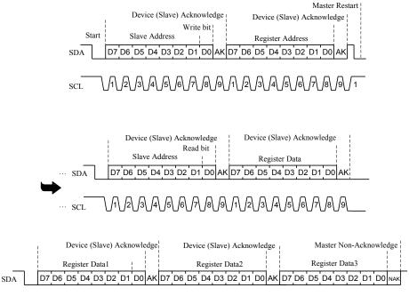
Figure 6: I<sup>2</sup>C Read Timing Diagram
