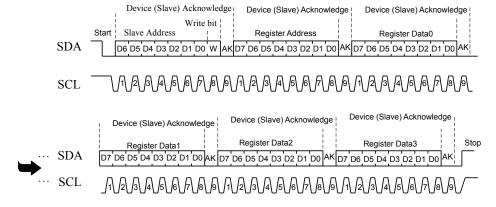
Figure 5: I<sup>2</sup>C Write Timing Diagram
