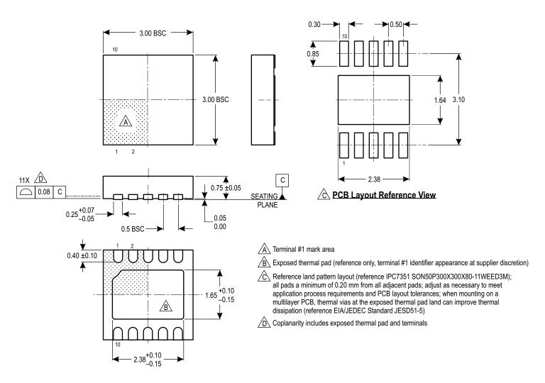
Figure 10: DFN10 (EJ) Package Drawing
