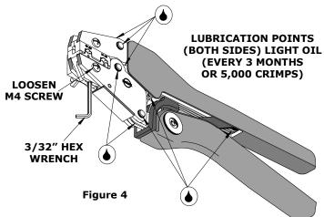
in Figure 4 every 5,000 crimps or 3 months will significantly enhance the tool life and ensure a stable calibration.
