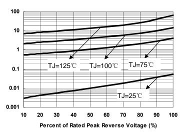
Fig.1-Typical Junction Capacitance
