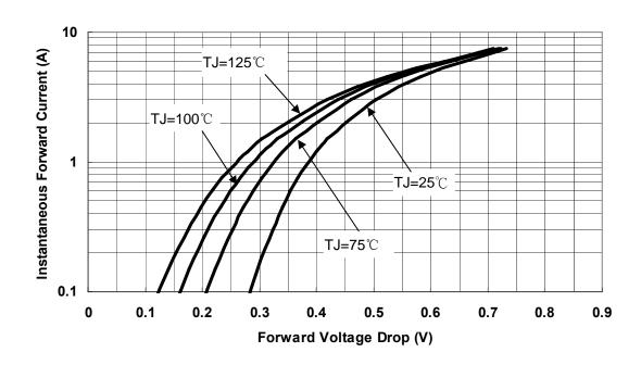
Fig.3-Typical Forward Voltage Drop Characteristics
